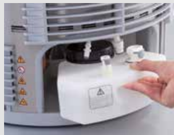
Installing media containers
