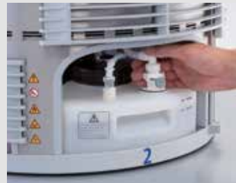
Connecting media containers
