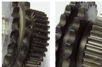
Removal of oil and swarf
